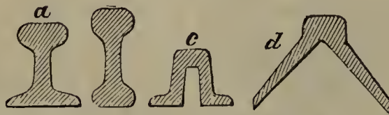
Cross Sections of Rails.
